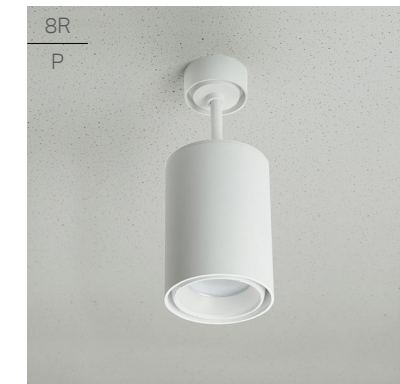
Wide Beam Reflector + Prismatic Lens 55° Beam, UGR16 / UGR19^, IP54
