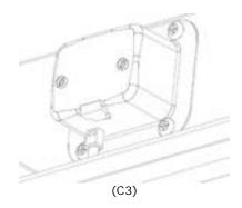
• In order to complete the replacement, remove the four screws and install the new module.
