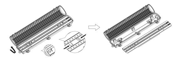
Step 4: Take the cable gland out and connect the AC cable.
