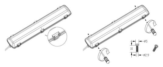
Step 7: Install the batten on the ceiling.
