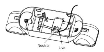
Connect AC wring cable to terminal block.
