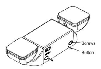
Remove the 2 screws from the unit, then press the button open the unit.
