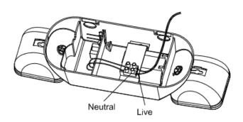
Connect AC wring cable to terminal block.
