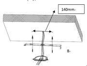
4. Connect the Power supply wires to the terminal block, select the colour temperature from DL/CW/WW using DIP switch.
