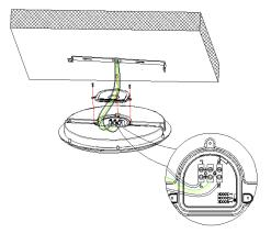
5. Fix the terminal cover with screws.
