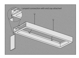
Lift out the end cap and let the end cap hang with the connected lanyard.
