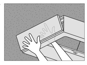
Remove one end cap on either side of the frame by pushing the end cap from the inside.
