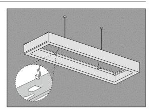
Bend the four frame suspension hole attachments to 90 degrees.
