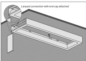
Remove one end cap on either side of the frame by pushing the end cap from the inside. Lift out the end cap and let the end cap hang with the
