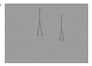
Switch off mains power. Fix suspension kit to ceiling. (Suspension kit not included).
